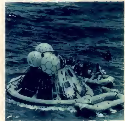
Recovery of Apollo Command Module after reentry. Note charring on heat shield from intense heat encountered during reentry into earth's atmosphere.
