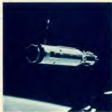
Agena docking vehicle, an unmanned spacecraft used by Gemini XII during historic first linkup of two vehicles in space.
