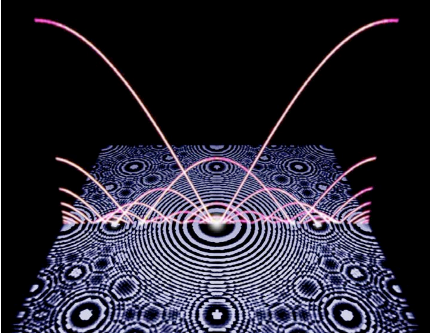
3.9. Cross-section of nonlinear standing waves (in pink) and their acoustic pressure distribution pattern (in blue)
