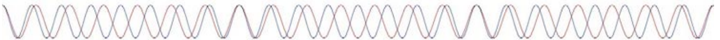
2.2. The interaction of two offset frequencies phasing in and out of synchrony to create an inaudible beat frequency
