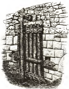
Drawing to show how the city gate might have been fastened to the bar-holds and the eye-bonder.
