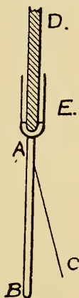
FIG. 24.—Working part of the above electroscopes, magnified four times. The rod AB with the gold leaf C is cemented to a thin rod of melted quartz D by means of a drop of mastic or guttapercha at the bottom of a minute metallic capsule E attached to the rod AB; thereby lessening any tendency of the charge to creep, and keeping the capacity exceedingly small.
